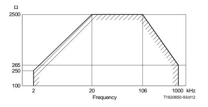
FIGURE 11/I.430 NT impedance template (log-log scale)
