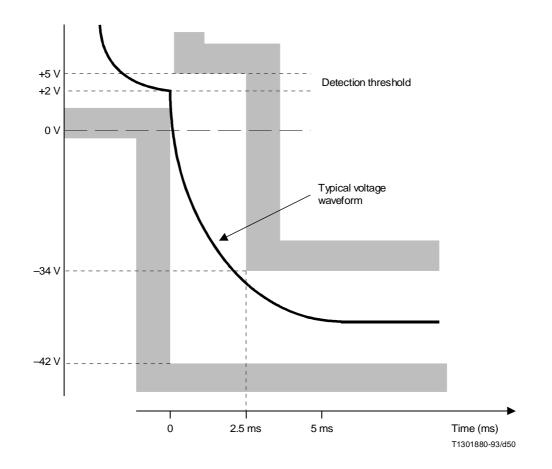
FIGURE 1.10/1.430 PS1 output voltage at switchover from APS
