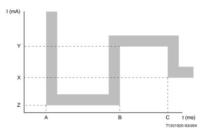
FIGURE II.1/I.430 TE current time mask (revised)
