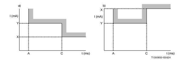
FIGURE 23/I.430 Current/Time limitation for TE
