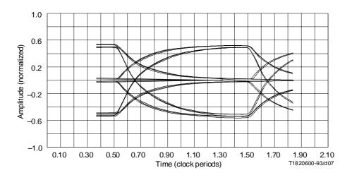
FIGURE 6/I.430 Waveform for test configuration i) – Point-to-point (6 dB) (C = 120 nF/km)
