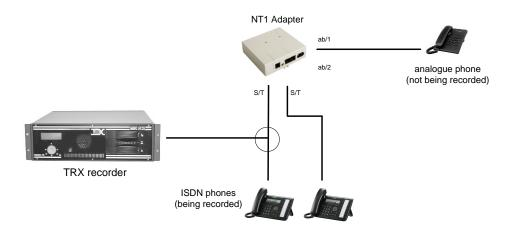
Recorder connected directly to the phone lineu
