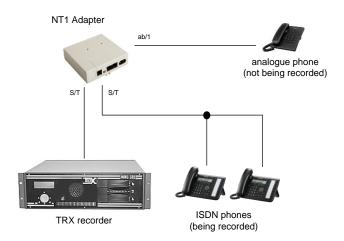
Recorder connected directly to the S/T socket in NT1 device
