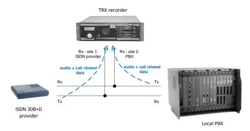
Connection of TRX recorder to an ISDN PRI line
