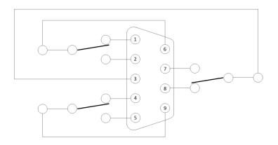
Position of the relays for alarm active or power failure
