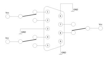
Position of the relays for alarm active
