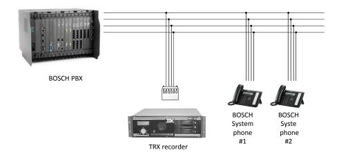
Connection recorder to BOSCH system line
